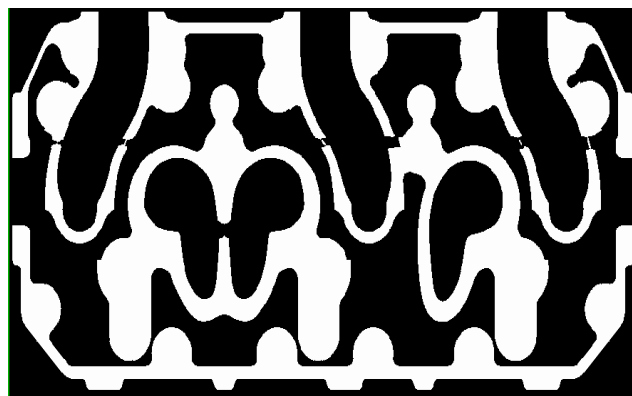
Fig.10. Central cylinder head projection after reconstruction by hull-voxel algorithm from truncated data and binary a priori supposal
