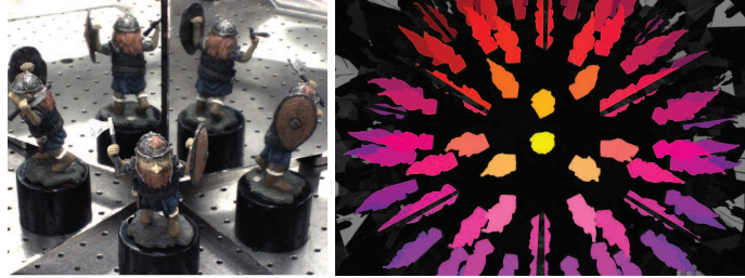
Fig. 17: The five-view case employing inter-reflections up to second order [25] – self-occlusion is clearly visible (left). In the case of many inter-reflections a pixel labeling procedure is necessary [2] that can resolve the view assignment to pixels – up to eight reflection levels have been employed (right).
